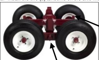
bolts and two (2) 1/4-20 x 2 1/2 bolts and two (2) 1/4-20 nuts. Make sure that the round tubes behind the wheels face upward. Position the nut underneath.
