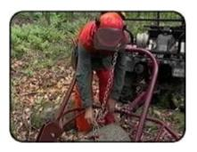
5. Start the ATV engine and skid the log. As the ATV moves forward, the log's weight tilts the arch and raises the log at the same time.
