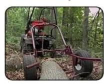
3. Tie the chain-choker and slide one link to one of the slots on top of the arch.
