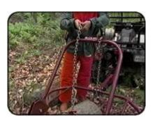
4. Hook the C-hook of the 3' (92 cm) tow bar chain to the chain-choker so that the hook slides freely.
