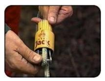
5. Hook the tow rope on the corner block. Attach the pulling plate on the ATV hitch and attach the cable to the plate with the clove hitch.
