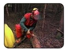
3. Thread the chain-choker through the opening of the skidding cone and position the cone on the top of the log to be skidded.
