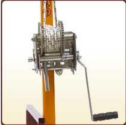
1. Fasten the winch handle to the winch with the nut provided. Then, fasten the winch to the loading mast with two (2) 3/8-16 x 2 1/2 bolts and two (2) 3/8-16 nuts.
