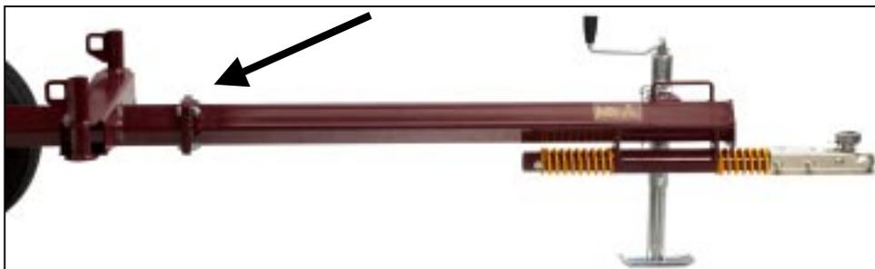
6. Install the protection grating (or the unloading mast support if you have the *Haul & Dump Kit*) on the front pole assembly with two (2) 1/2-13 x 4 carriage bolts and two (2) 1/2-13 nuts. Position the grating about **12" (30 cm)** of the assembly joint.
