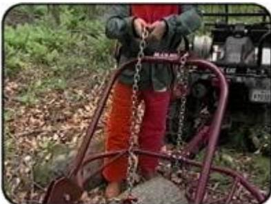
**4. Hook the C-hook of the 3' (92 cm) tow bar chain to the chain-choker so that the hook slides freely.**
