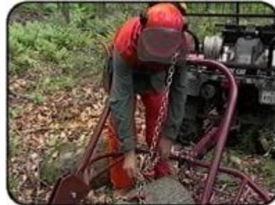
**5. Start the ATV engine and skid the log. As the ATV moves forward, the log's weight tilts the arch and raises the log at the same time.**
