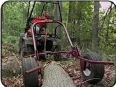
**3. Tie the chain-choker and slide one link to one of the slots on top of the arch.**
