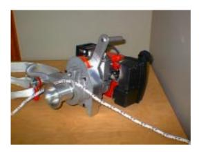
C. Wrap the rope around the rotating drum (3 loops).
